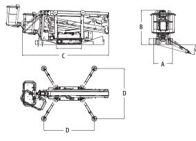
A. Stowed Width (without platform): B. Stowed Height (on tracks): C. Stowed Length (on tracks): D. Outrigger Footprint: 0.80 m 1.99 m 5.00 m 2.92 m x 2.93 m
